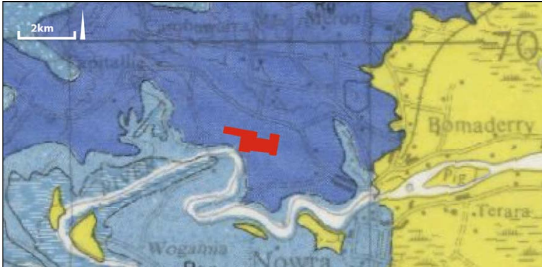
Figure 3. Wollongong 1:250 000 Geological Map showing the location of Lot 24 (red shading) on undifferentiated Berry Formation siltstone, shales and sandstone of the Shoalhaven Group soil landscape.
